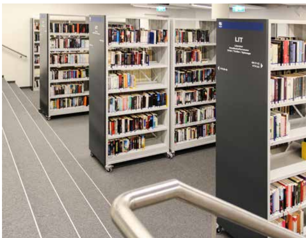
Library shelves with a moveable base can be pushed to the side to make room for events.
